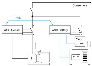
To improve power quality, the ASC-4 Battery can supply peak loads while gensets start. The ASC-4 Battery controller can support the load, so that the genset can run at its optimal load point. If the ESS is designed to supply the busbar load, the ESS can be the only source connected to the busbar.
