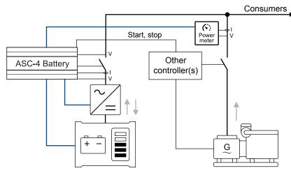
The ASC-4 Battery controller can support the load, so that the genset can run at its optimal load point.
